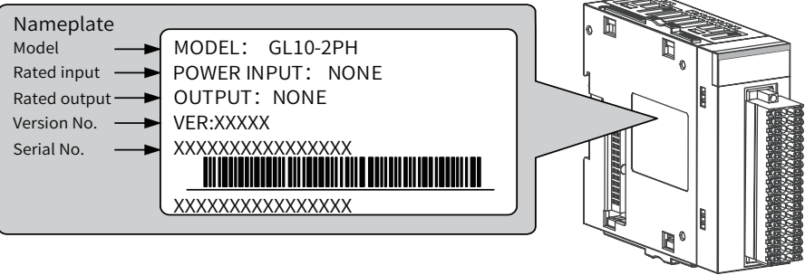
Figure 1 Description of model number and nameplate
