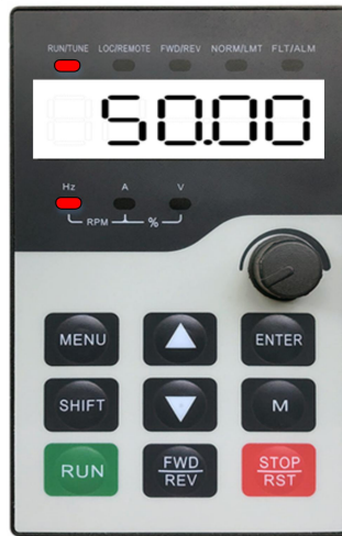
Figure 4-7 Steady operation of the frequency converter
