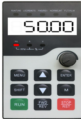
Figure 4-6 Frequency converter power-on display
