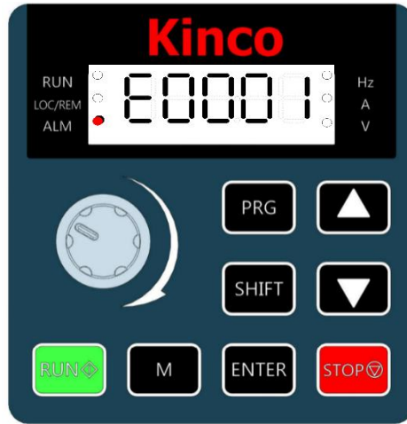
Figure 6-1 The interface fault display
