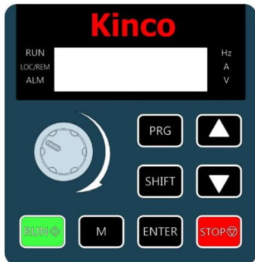
Figure 4-1 Schematic diagram of the LED operating panel
